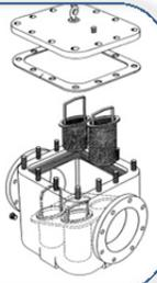
Strainer chamber covers can be secured to the strainer body with studs/nuts or a "quick opening" style that does not require tools to open the basket chamber, such as a yoke style clamp, swing bolts or knobs.
