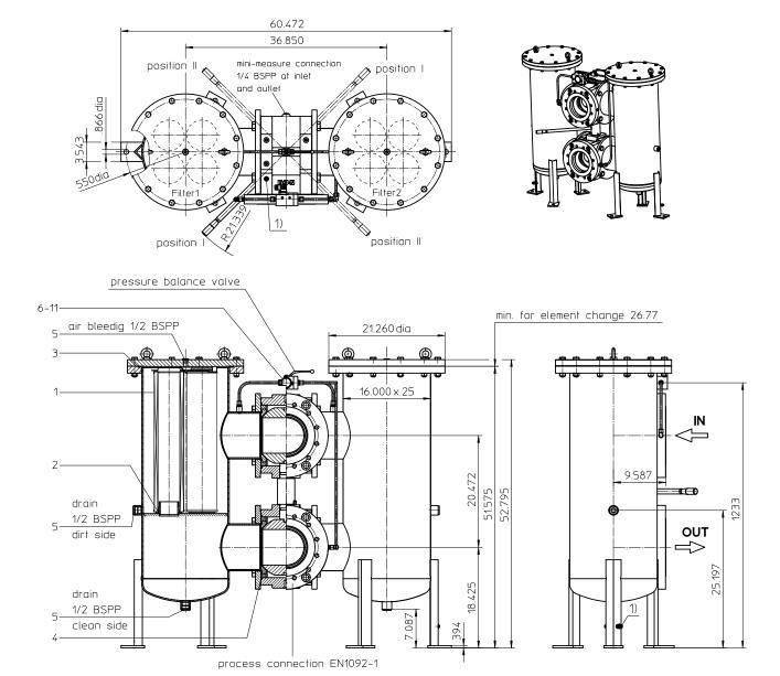
Position I: Filter 1 in operation Position II: Filter 2 in operation
