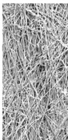
The LOFCLEAR 500 has a fully welded design to maintain flow path integrity as well as ensuring the strength of the filter bag to reduce the chance of rupture as it can hold just over 2 lbs. of particles. The outer layer consists of a fine mesh to prevent fiber migration of the meltblown fibers of which the filter bag is constructed. The polypropylene fibers used in the melt blown
