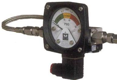
Monitoring your differential pressure is especially important for retention of gel-like particles as they are more likely to deform and pass through your filter media at higher differential pressures. Thus, a consequence of gelatinous particle filtration is increased frequency of element cleaning or replacement.
