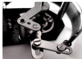
Welding style and quality equally applies at the closed end of the Bourdon tube, where the linkage is attached. A pivot
