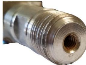
The pressure gauge socket (inlet) is the first part of the gauge the process fluid contacts, unless you are isolating it with a diaphragm seal.
