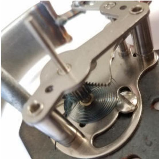
The pointers themselves vary in complexity. Some like the one picture here enable fine adjustments to compensate for altitude or wear caused by pulsations and vibration.
